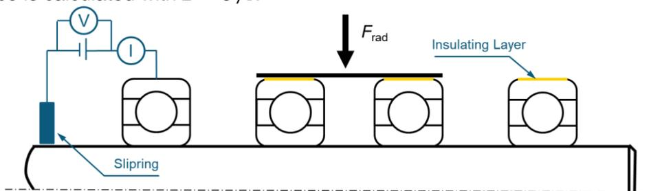
Figure 4: Bearing test bench
