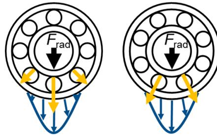
Figure 3: The two extreme states of roller position in roller bearings
