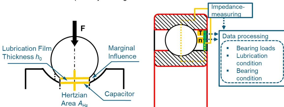
Figure 1: The rolling contact modelled as a capacitor depending on lubrication film thickness and Hertzian area
