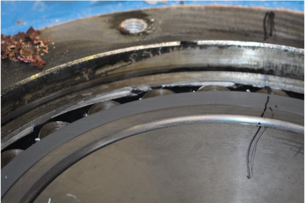
Figure 4: propagated bearing damage leading to ring fracture, misalignment of the shaft and subsequent gearing damage
