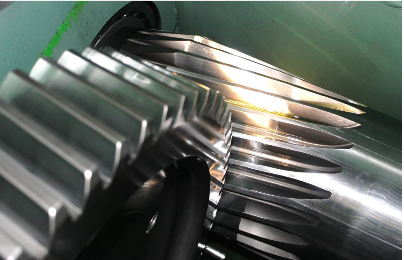
Figure 6: typically, gears can be inspected completely if the input shaft can be turned slowly
