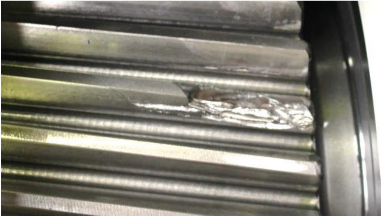
Figure 2: fatal gearing damage
