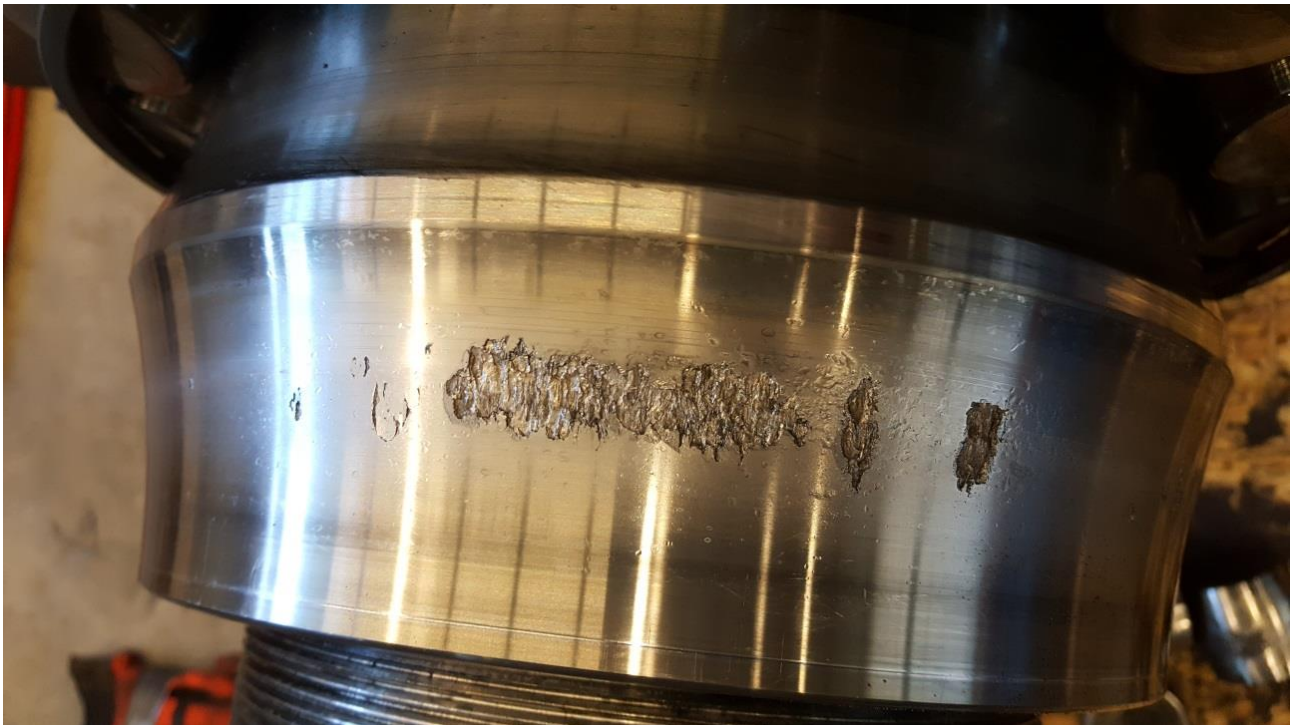
Figure 3: early stage bearing damage
