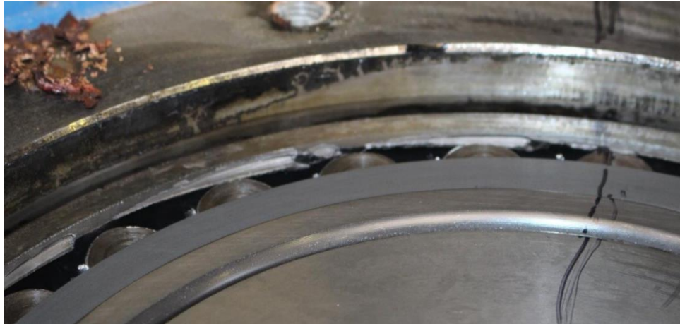
Figure 2: (a) Early-stage bearing damage (localized spalling); (b) Late-stage bearing damaged (widespread spalling propagation and resultant ring fracture)
