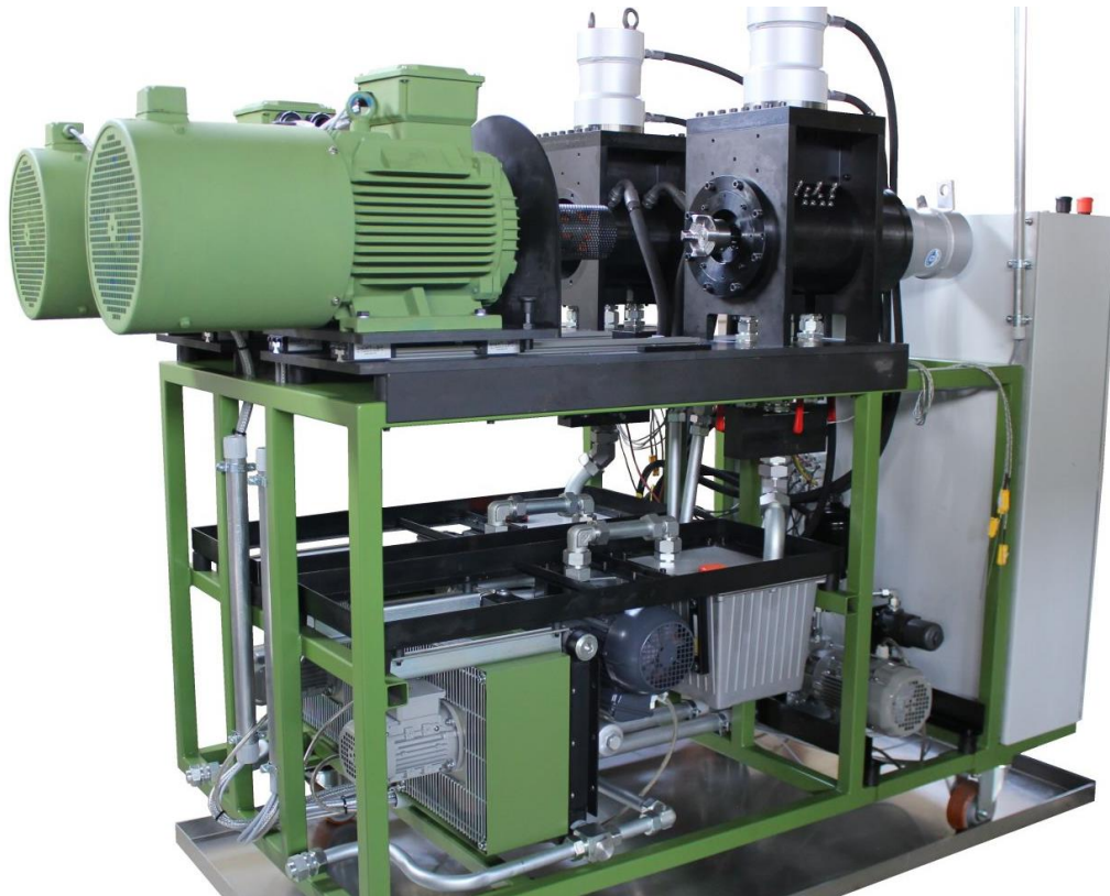
Figure 3: An EELPRAAX-130 test rig for bearings up to 130mm outer diameter under axial, radial, or combined loads.
