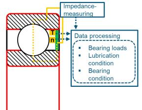
Figure 2: Load sensing bearing with insulating layer (red), connector (green), current flow (yellow) temperature (T) and rotation speed (n) sensor
