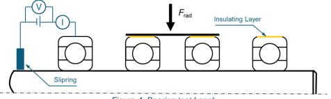
Figure 4: Bearing test bench
