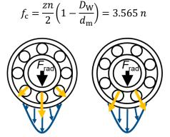
Figure 3: The two extreme states of roller position in roller bearings
