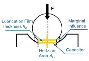
Figure 1:The rolling contact modelled as a capacitor depending on lubrication film thickness and Hertz'ian area
