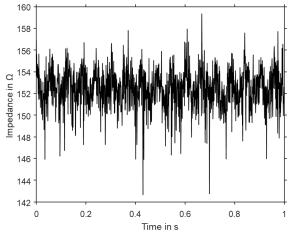
Figure 5: Measurement of the electric bearing impedance
