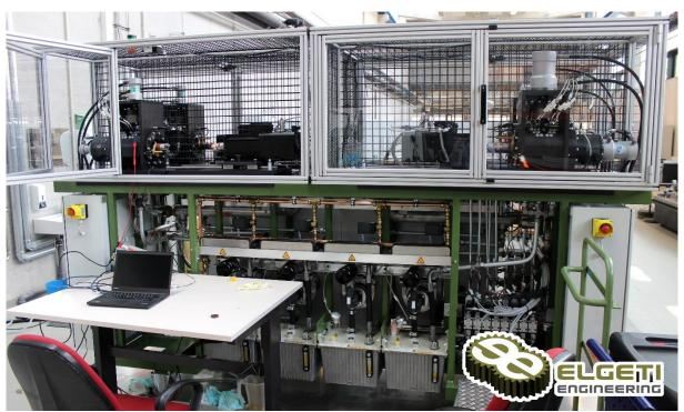
Figure 8: EELPRAAX-80-4E bearing test rig by Elgeti Engineering GmbH
